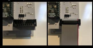
While the case is powered down, plug the other end of the ribbon cable into a 16pin power output connector on the power supply of the case. Make sure that the ribbon cable is oriented so that the red strip is on the side of the connector that supplies -12v. On many cases the -12v side of the connector is labeled with a stripe. Screw the module into the case and power on the case. At this point you should see the light on the module begin to blink.
