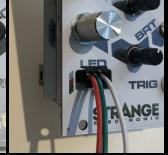
The LED strip has two connectors on it. One is for plugging in the LED extension cable and the other one is for plugging in the 5v power supply.
