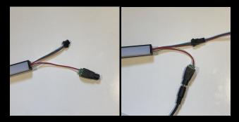
Be sure that you only plug the provided 5v power supply into the LED strip. Plugging in a power supply with more than 5 volts will break the LEDs. So as a safety precaution, check the voltage of the power supply before plugging it in. To do this look on the bottom of the body of the power supply and make sure it says 5v - 5a as shown in the picture below.
